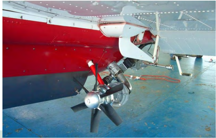
Right: Air Tractor AT-802F fitted with spray pump beside the computerized fire fighting door
