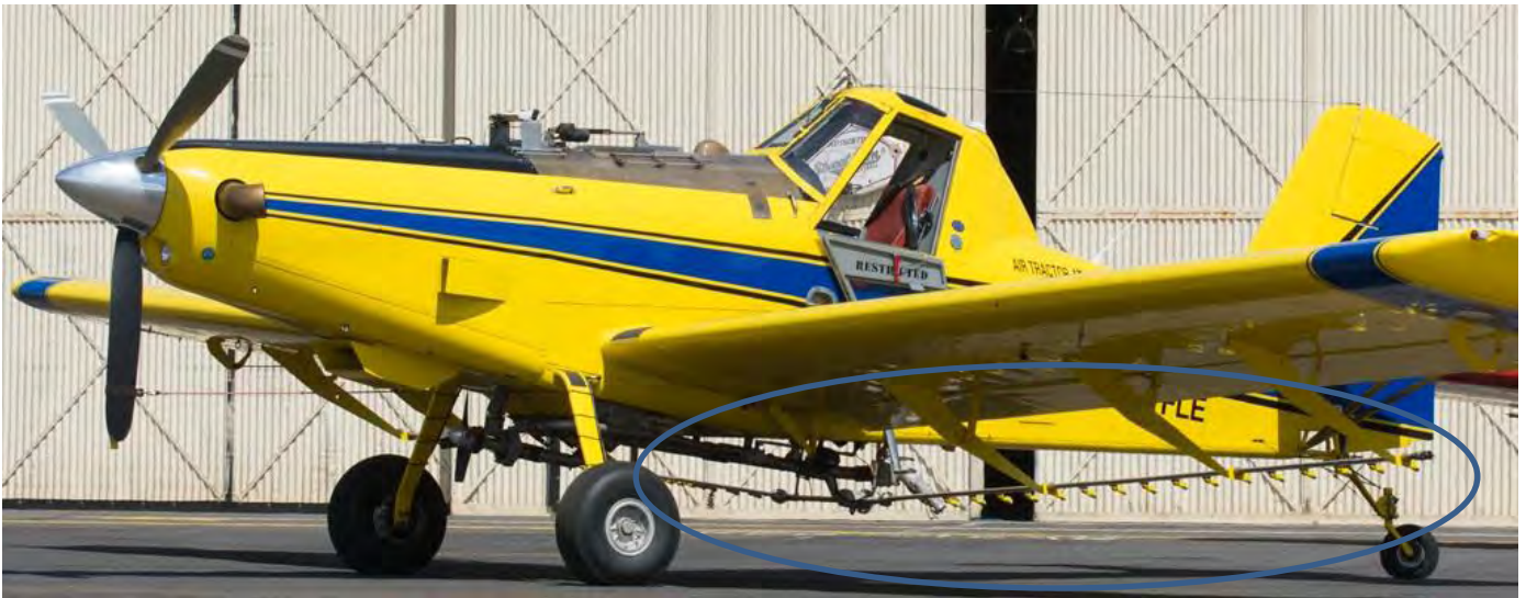
Above: Air Tractor AT-402B fitted with spray pump and spray booms for morning spray operations
