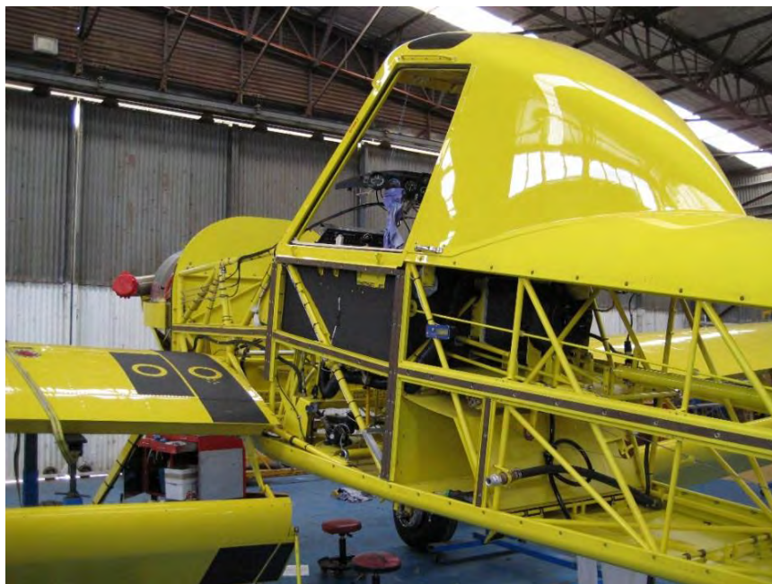
Air Tractor AT-504 – in process of reassembly in Australia
