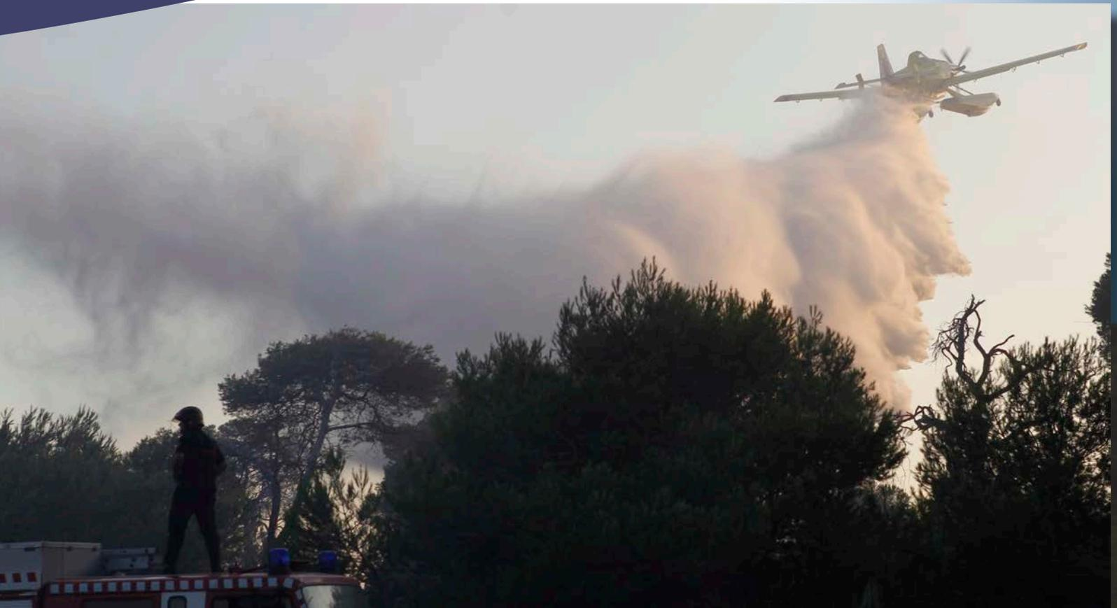
The Fire Boss can quickly climb to high mountain elevations and execute aggressive down-slope drops.
